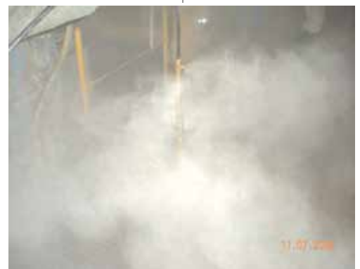
Test work was required to clarify the performance of the fogger system for suppressing respirable silica dust
