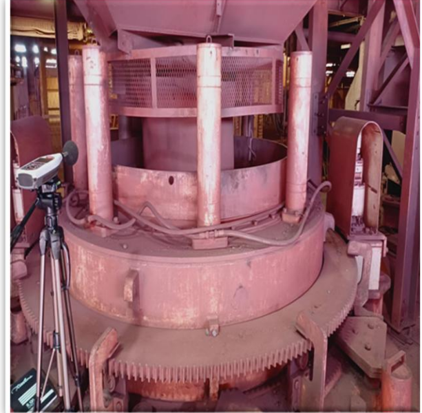
Feeder level noise measurements in progress
