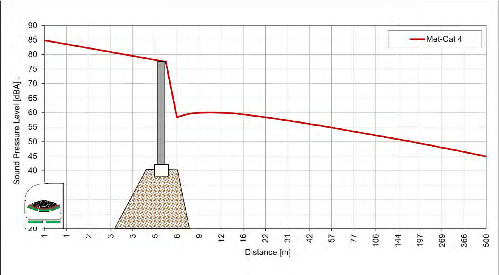
Effect of Screen on Conveyor Noise Level
