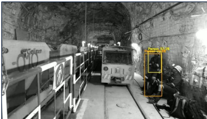
Pedestrian Posture – Detection of leaning pedestrian
