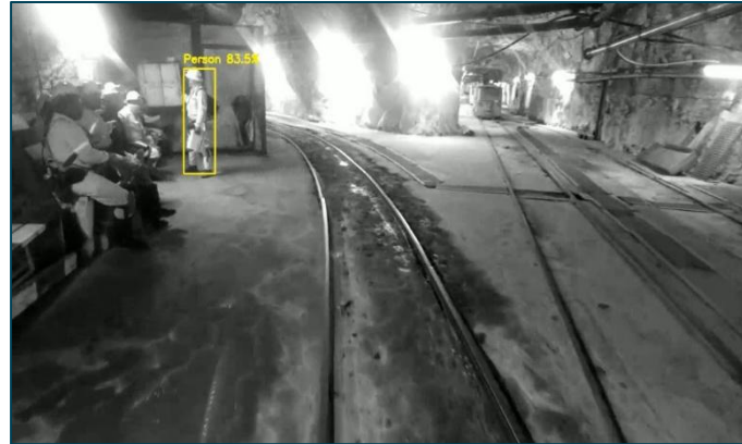
Multiple pedestrians – First pedestrian detected
