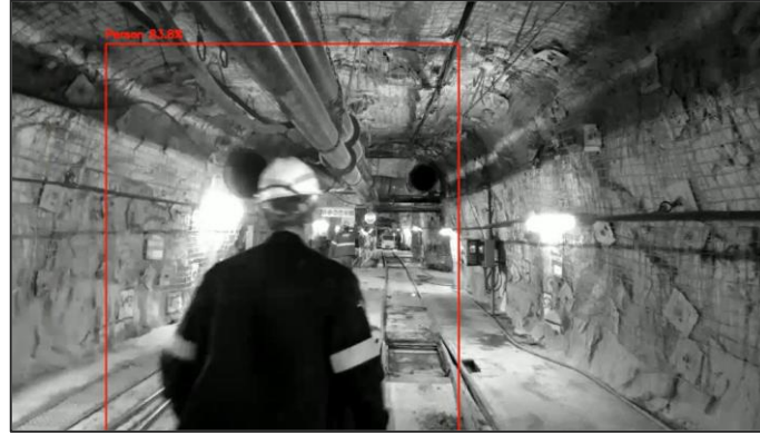
Pedestrian walking away – Detection 0-5 meters
