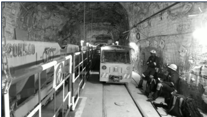
Pedestrian Posture – No detection for leaning and sitting pedestrians
