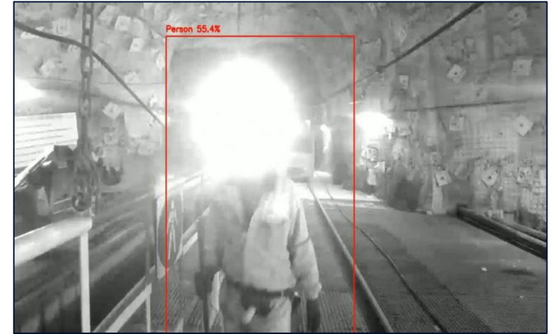
Pedestrian with cap lamp – Tracking resumes, super slow zone
