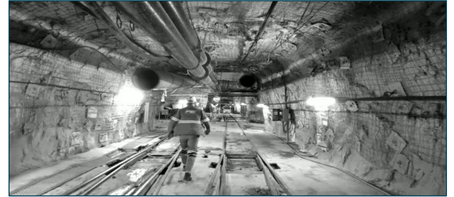
Pedestrian walking away – Detection, presence 15-20 meters
