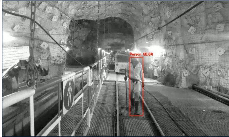
Pedestrian with cap lamp – Tracking continues into super slow zone
