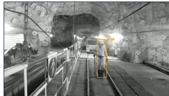
Pedestrian with cap lamp – Tracking resumes, slow zone
