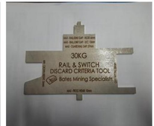
MAX - RAILJOINT GAP - PLCE: 6mm MAX - RAILJOINT GAP - JWC: 15mm MAX - GUARD RAIL GAP: 57mm 22KG RAIL & SWITCH DISCARD CRITERIA TOOL Bates Mining Specialists MIN. CHAIN WELD: 20mm DON. WIDTH: 40mm MAX - TROG WEAR: 10mm
