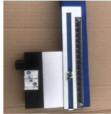
MAX - RAILJOINT GAP - PLCE: 6mm MAX - RAILJOINT GAP - JWC: 15mm MAX - GUARD RAIL GAP: 57mm 22KG RAIL & SWITCH DISCARD CRITERIA TOOL Bates Mining Specialists MIN. CHAIN WELD: 20mm DON. WIDTH: 40mm MAX - TROG WEAR: 10mm
