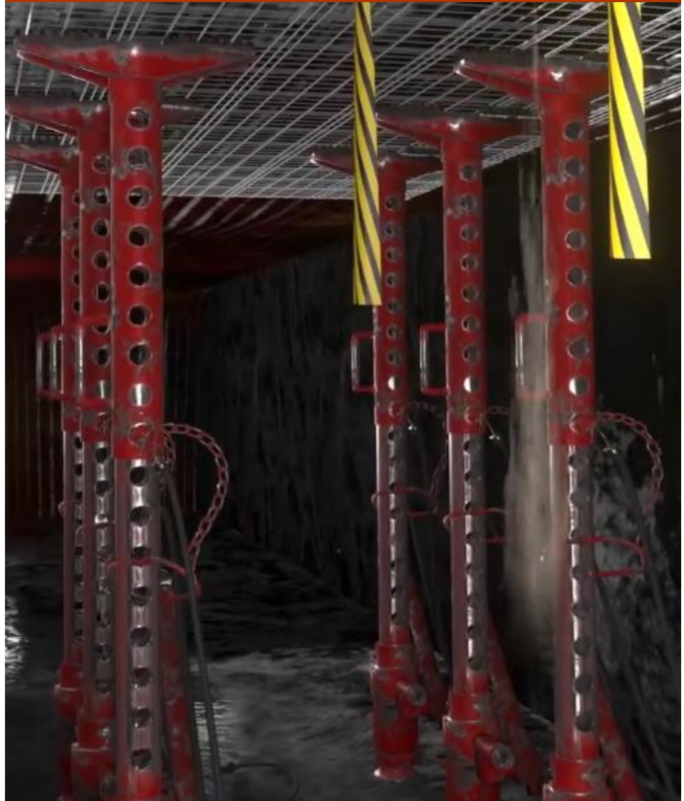
Suspension of roof welded mesh with hydraulic/ temporary support jacks
