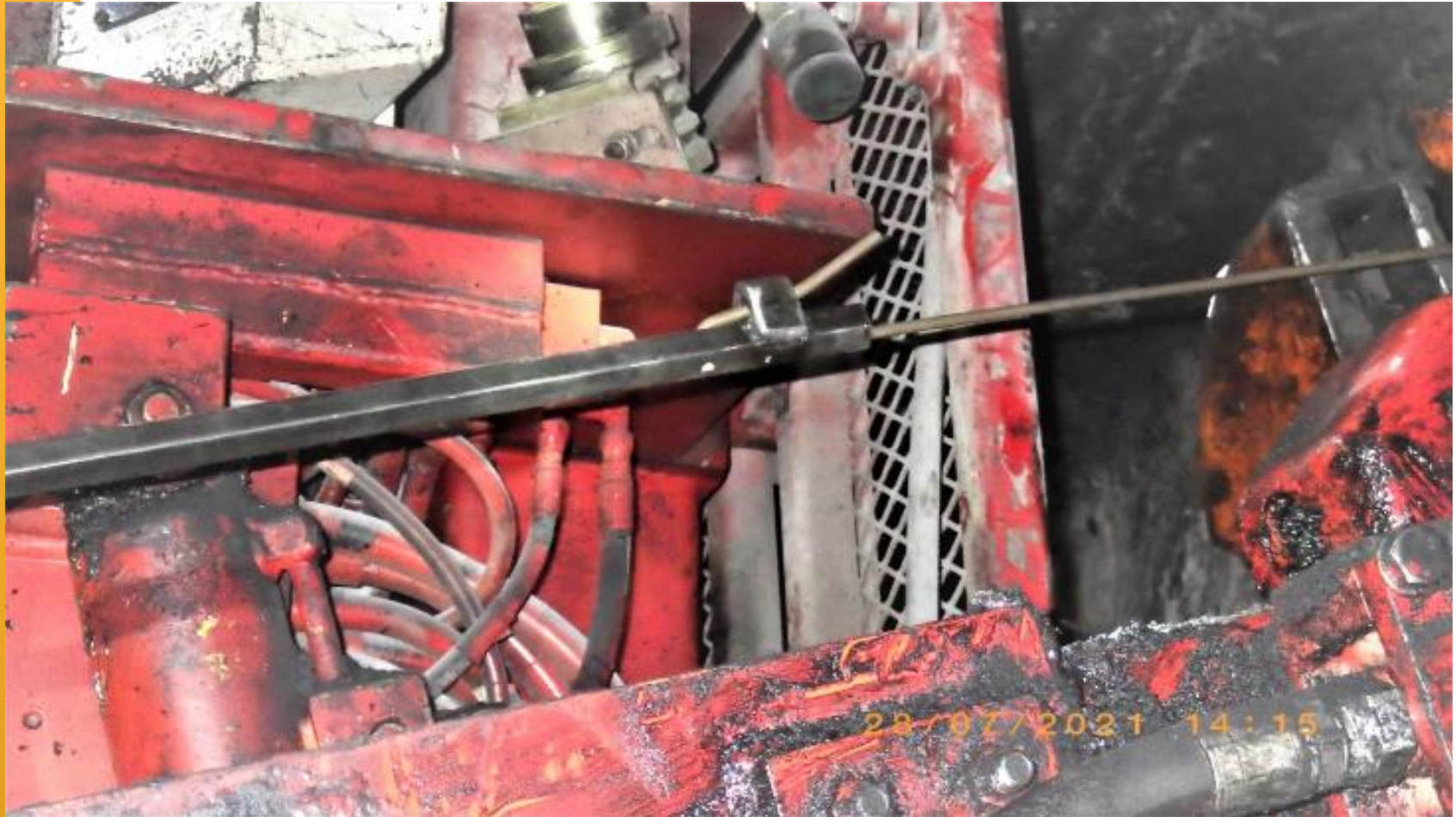
Image 3: Z-Hook and insertion tool in roof bolter chuck, ready to insert Z-Hook.
