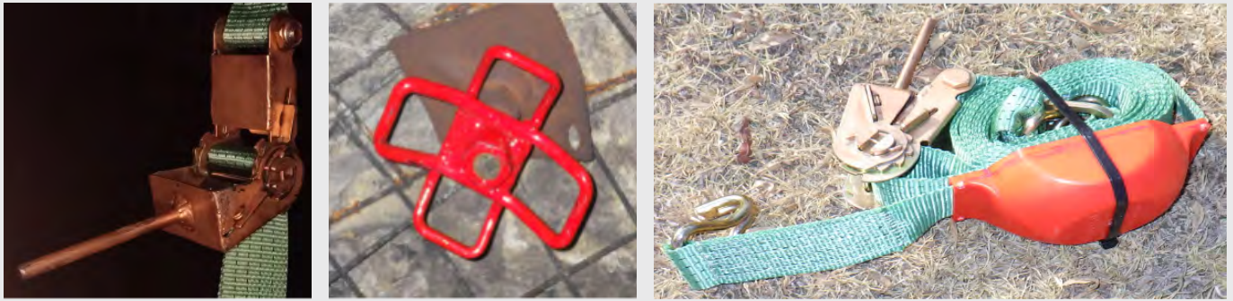
Figure 2: DTM Strap used for strapping loaded mesh
