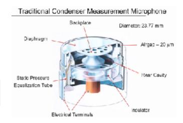
A microphone is distinguishable by the voltage value produced when a known, constant root mean square sound pressure is applied. This is known as microphone open-circuit sensitivity.
