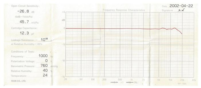
Each microphone's manufacturer's calibration certificate shall be filed, not just for comparison evaluation for the calibration laboratory testing the open-circuit sensitivity of the microphone but also for the purpose of history and drift of the microphone.
